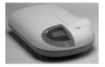
Estimation of the concentration of solutions by spectrophotometry is possible because the quantity of light absorbed by the particles in a solution, or the optical density (O.D.), increases linearly with concentration. A light beam is shone through the solution question and light in absorption is detected using a photosensitive element which reads out optical density (or the log of its percent inverse, light "transmittance") on an appropriately calibrated meter scale.
