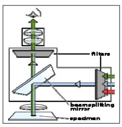
**Confocal Scanning Microscope**: Confocal Laser Scanning Microscopy (CLSM) is an optical microscopy technique that is based on conventional wide-field fluorescence microscopy. The use of modern technology (laser, photomultiplying detectors) in CLSM gives this method a lot of advantages. The laser beam is focussed into the sample and by using electronic lenses and apertures only the fluorescence light that comes directly from the confocal plane is detected by a photomultiplier.
