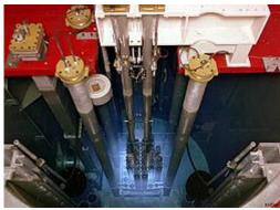
Blue <u>Cherenkov radiation</u> light being emitted from a <u>TRIGA reactor pool</u> is due to high-speed beta particles traveling faster than the speed of light (phase velocity) in water (which is 75% of the speed of light in vacuum).
