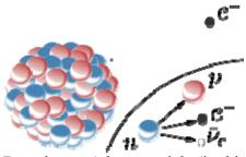
Beta decay. A beta particle (in this case a negative electron) is shown being emitted by a <u>nucleus</u>. An antineutrino (not shown) is always emitted along with an electron. Insert: in the decay of free neutron, a proton, an electron (negative beta ray), and an <u>electron</u> <u>antineutrino</u> are produced
